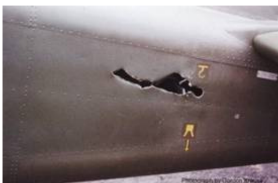
Note the damage and the lift/tie down symbol.
